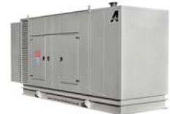
500kVA zintec steel generator canopy silenced to 60dB(A) @ 1 metre
